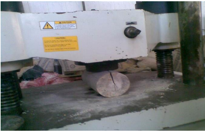
Figure 11: Image of failure after the Brazilian test on plain concrete cylinders
