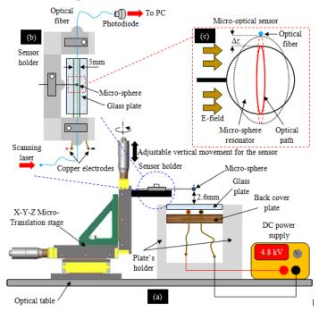
Fig. 2. A schematic of the experimental setup based on the Whispering Gallery Modes, where (a) is the X-Y-Z Micro-Translation stage, (b) is the sensor holder in the form of a C-shape and (c) is the micro-optical sensor.
