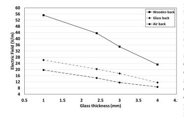
Fig. 4. The electric field above a glass surface as a function of the glass thickness and the back cover material; wood, glass and no cover, i.e. air.
