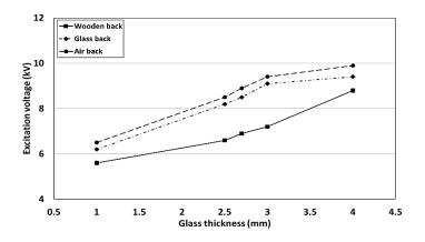
Fig. 7. Influence of glass thickness and the electrodes back cover material on the excitation voltage of the electrostatic cleaning system. The diameter of the electrodes is 0.16 mm and the pitch of the electrodes is 2 cm.
