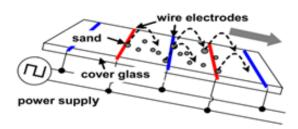
Figure 1. Schematic diagram of the enhanced system that removes dust particles under the influence of standing wave generated by single phase rectangular high voltage power supply and gravity [15].
