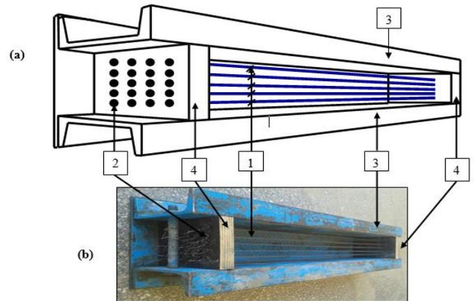
**Fig. 3.** (a) Sketch and (b) photo of installation of continuous steel fibers of SI-CSFRC beam. (1) Continuous steel fibers, (2): clamping screws, (3) steel mold, and (4) perforated wooden plate.
