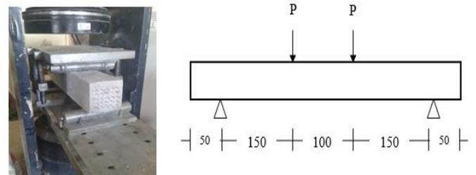
**Fig. 5.** Experimental set-up and two-point loading arrangement, all dimension in mm.
