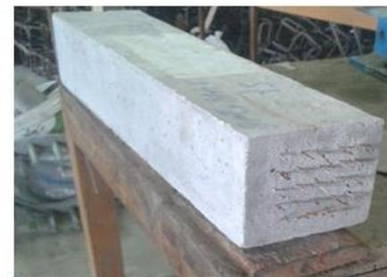
**Fig. 4.** Demolded single inline-continuous steel fiber reinforced concrete (SI-CSFRC) beam.
