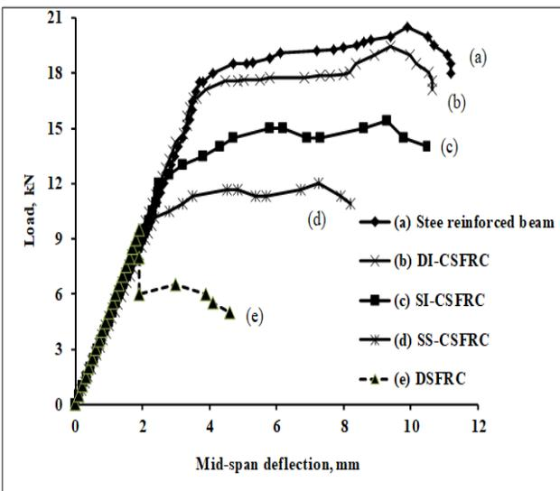
**Fig. 6.** Load – deflection behavior of (a) steel reinforced beams, (b) DI-CSFRC, (c) SI-CSFRC, (d) SS-CSFRC, and (e) DSFRC beams.
